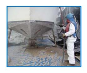
The boat's fairing maintenance is something that cannot be avoided in order to protect it from corrosion (for metals), musty and rot (for woods), osmosis (for plastics) and especially from aquatic organisms' settlement, which, if passively transported to different microclimatic environments, could also easily colonise them invasively.
