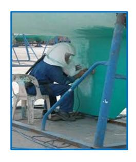
Ten's thousands tons of extremely toxic "antivegetative" coating (or anti-fouling paint) are used every year to protect the boat hull from sea organisms (algae, shellfish...). Remember that each kg of antifouling paint normally contains 70 g of biocides, of which 1 g is enough to pollute several m3 of seawater, and also that the necessary PPE must be worn as it is toxic.
