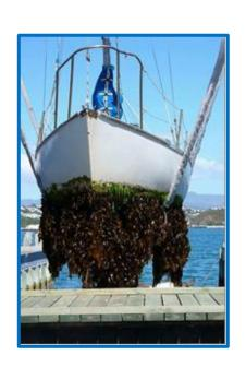
"Fouling" is a natural phenomenon that emerges with the formation of an invisible biofilm, which is rapidly colonized – according to light, temperature and nutrient richness of the water - by parasitic organisms. Unfortunately, the fairing of a boat shell is critical because a smooth hull offers less resistance to movement, increasing boat speed and reducing its fuel consumption (1 to 2 mm of algae or organisms fixed on a shell causes a 15% loss of speed).
