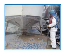
The boat's fairing maintenance is something that cannot be avoided in order to protect it from corrosion (for metals), musty and rot (for woods), osmosis (for plastics) and especially from aquatic organisms' settlement.
